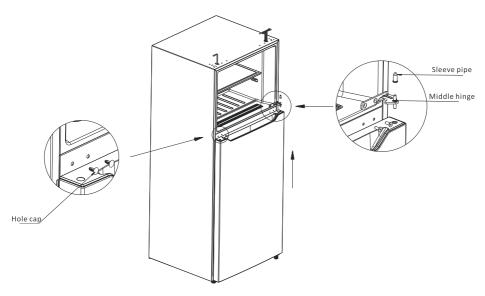
4)Dismantle the lower hinge assembly and levelling foot C, then dismantle the sleeve pipe and hinge shaft, move levelling foot B to right hole, Install the hinge shaft and sleeve pipe to the left hole of lower hinge, and then install the lower hinge assembly to the lower left corner of the refrigerator. Finally, install the levelling foot C to the lower right corner of the refrigerator.
