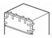
2)Please dismantle the fitting screws of top cover, and lift the top cover up a little, then disconnect the connection of signal line A and B, take out the sensor, and separate the right hinge cover from top cover; disconnect the connection of signal line E and D, then remove the fitting screws of right hinge and remove the freezer door.
